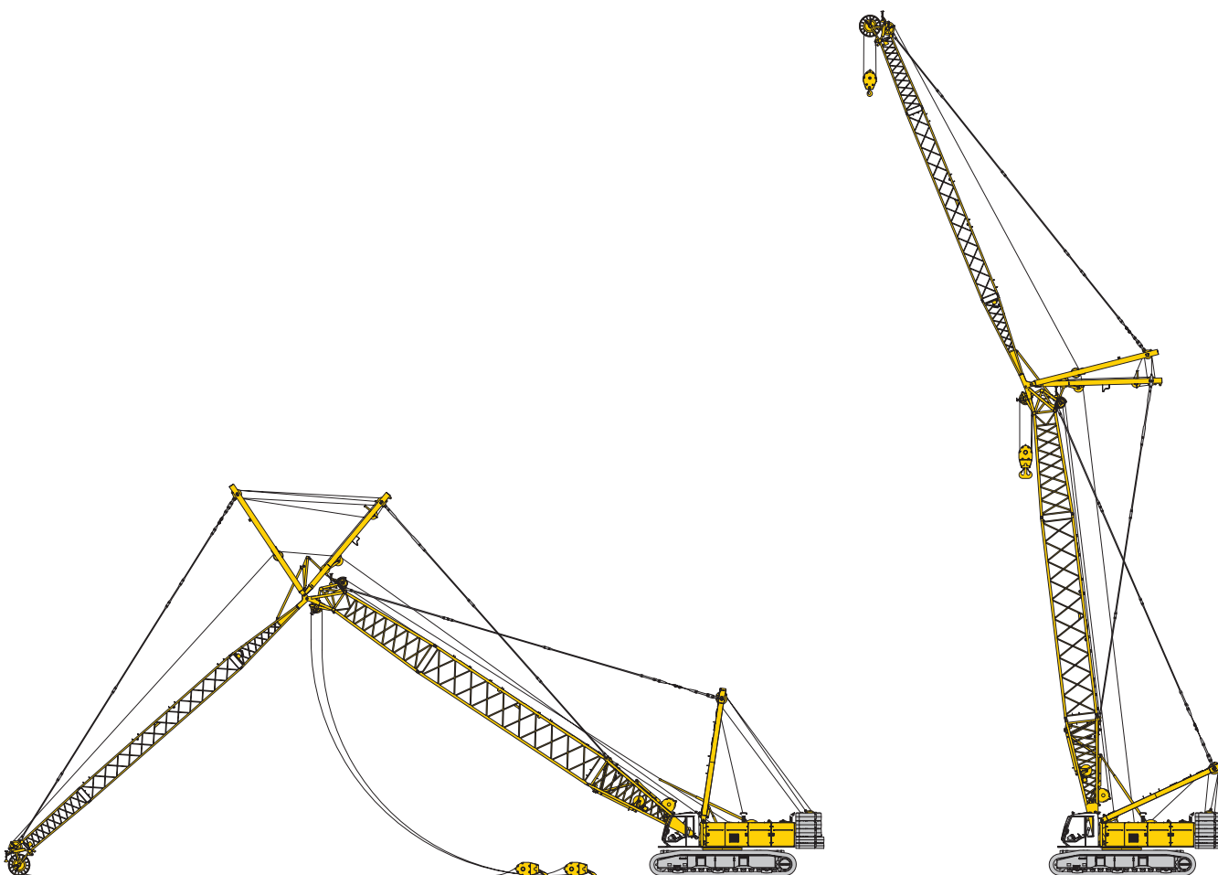
Erecting of main boom and luffing jib
